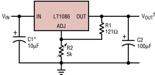
\*NEEDED IF DEVICE IS FAR FROM FILTER CAPACITORS
