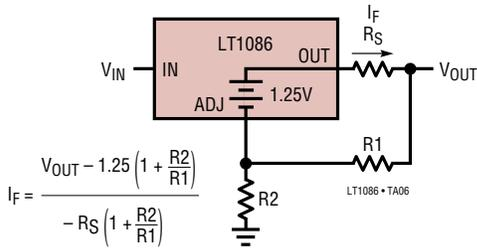
$$I_F = \frac{V_{OUT} - 1.25 \left(1 + \frac{R2}{R1}\right)}{-R_S \left(1 + \frac{R2}{R1}\right)}$$
