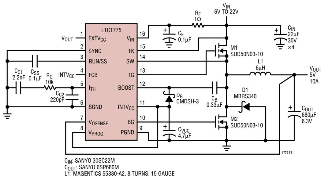
Figure 11. 5V/10A Fixed Output from Design Example
