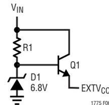
Figure 6. EXTV<sub>CC</sub> Power Supplied from  $V_{IN}$
