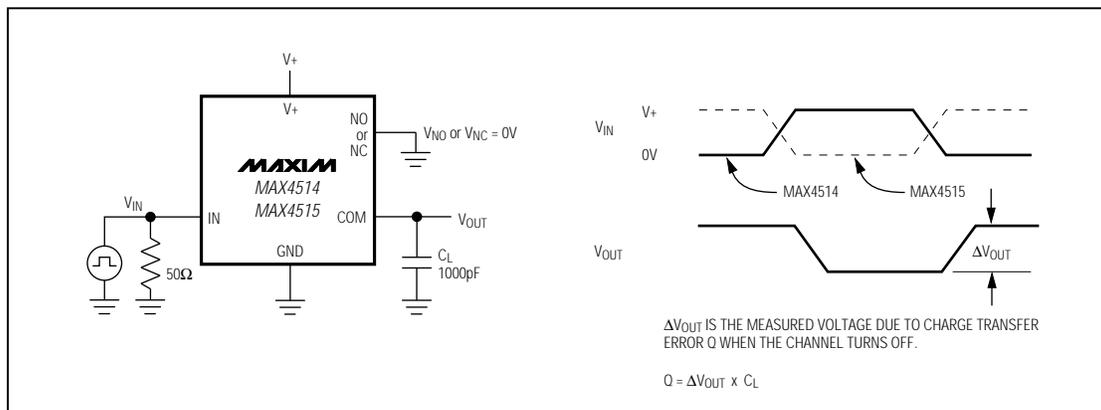
Figure 1. Charge Injection
