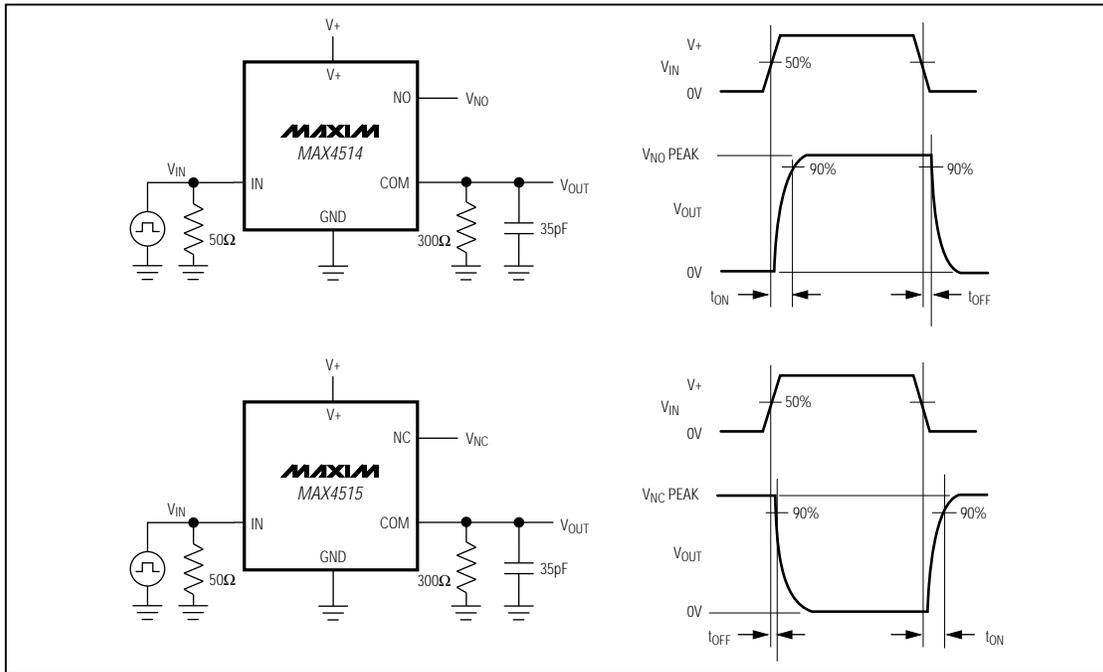
Figure 2. Switching Times
