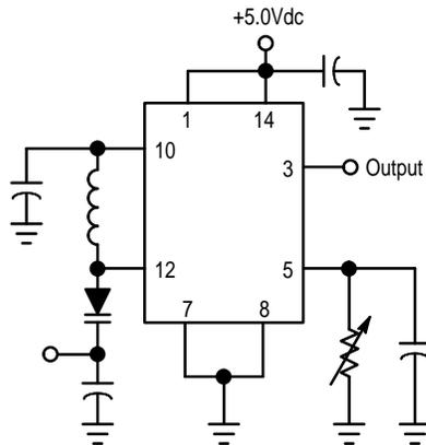
Figure 10. Method of Obtaining a Sine-Wave Output
