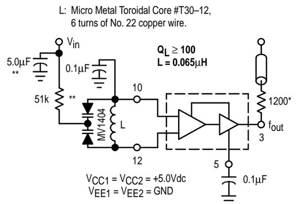
\* The 1200 ohm resistor and the scope termination impedance constitute a 25:1 attenuator probe. Coax shall be CT-070-50 or equivalent. NOT used in normal operation.
