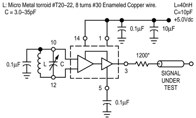
\* The 1200 ohm resistor and the scope termination impedance constitute a 25:1 attenuator probe. Coax shall be CT-075-50 or equivalent.
