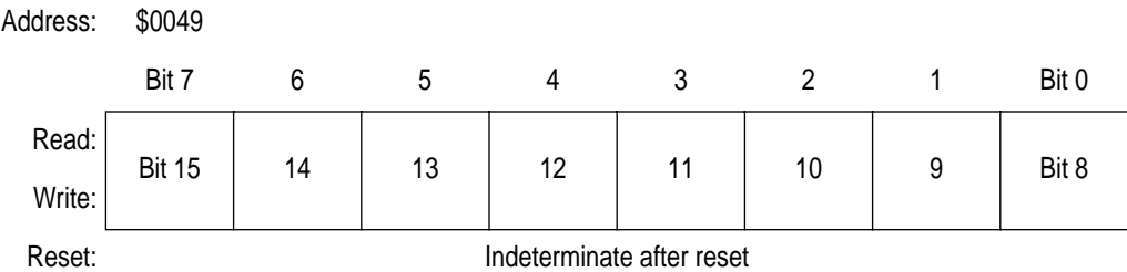
Figure 12-16. TIMB Channel 1 Register High (TBCH1H)
