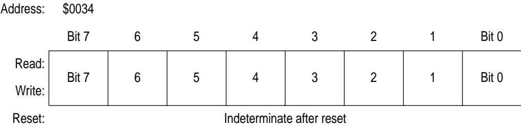
Figure 12-19. TIMB Channel 2 Register Low (TBCH2L)
