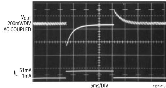
Figure 11b. Inclusion of a 100k/22nF Series RC on  $V_C$  Pin Results in Overdamped Stable Response
