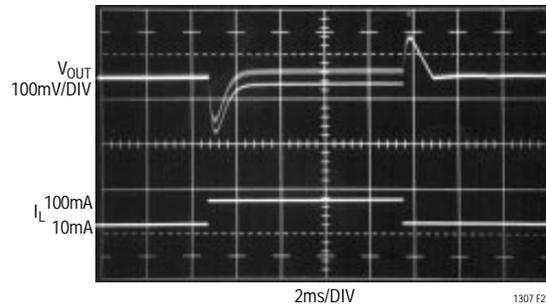
This photo shows transient response in constant switching mode with a 10mA to 100mA stepped load. Output ripple at the switching frequency can be reduced considerably by adding a 10µF ceramic capacitor in parallel with the 100µF tantalum.
