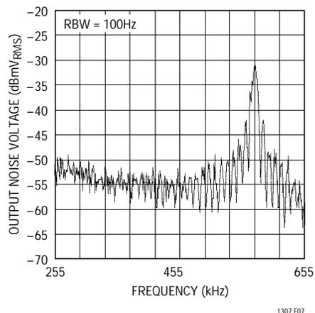
Figure 7. Span Centered at 455kHz Shows  $-55dBmV_{RMS}$  (1.8 $\mu$ V<sub>RMS</sub>) at 455kHz. Burst Mode Creates Sidebands 5.1kHz Apart Around the Switching Frequency Fundamental of 575kHz
