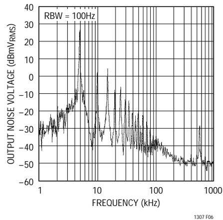
Figure 6. Spectral Noise Plot of 3.3V Converter Delivering 5mA Load. Burst Mode Fundamental at 5.1kHz is 23dBmV<sub>RMS</sub> or 14mV<sub>RMS</sub>
