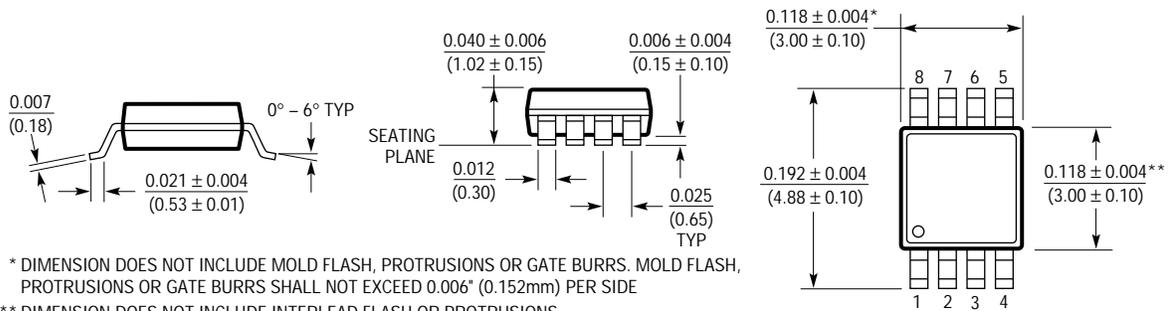
\* DIMENSION DOES NOT INCLUDE MOLD FLASH, PROTRUSIONS OR GATE BURRS. MOLD FLASH, PROTRUSIONS OR GATE BURRS SHALL NOT EXCEED 0.006\* (0.152mm) PER SIDE
