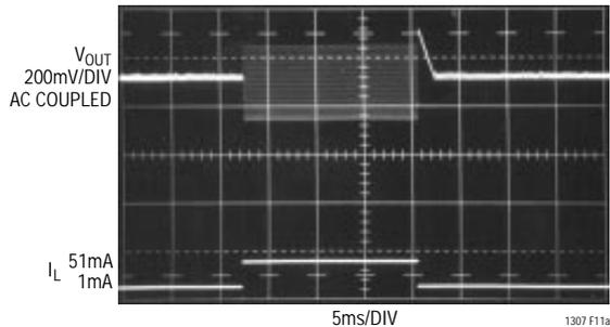
Figure 11a.  $V_C$  Pin Left Unconnected. Output Ripple Voltage is 300mV<sub>P-P</sub> Under Load
