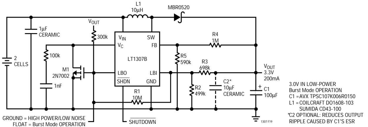
This circuit overcomes the limitation of load-based transitioning between Burst Mode operation and constant switching mode by adding external control. If M1's gate is grounded by an external open-drain signal, the converter functions normally in constant switching mode, delivering 3.3V. Output noise is low, however efficiency at loads less than 1mA is poor due to the 1mA supply current of the LT1307B. If M1's gate is allowed to float, the low-battery
