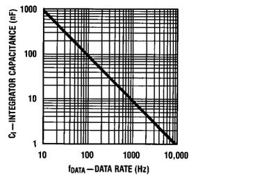
FIGURE 21. Impulse noise filter cap.  $C_I$  versus  $f_{DATA}$  where the charge time is  $\frac{1}{2}$  bit time
