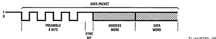
FIGURE 32. A simple encoded data packet, generated by the transmit controller is shown. The horizontal axis is time where 1 bit time is  $1/(2f_{DATA})$
