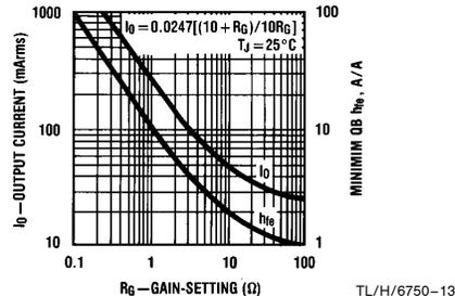
FIGURE 11. Output amplifier current and required min. Q<sub>B</sub> h<sub>fe</sub> versus gain-setting resistor R<sub>G</sub>
