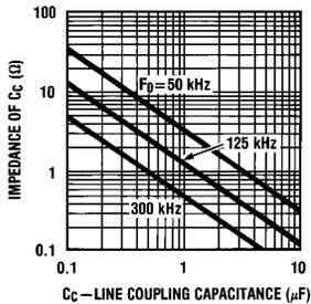
FIGURE 9. C<sub>C</sub>'s impedance should be, as a rule-of-thumb, smaller than the lowest expected line impedance
