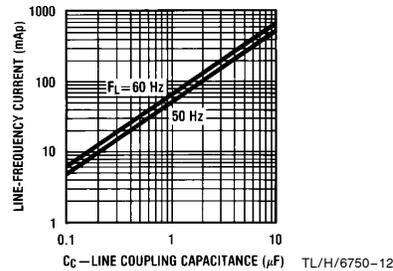
FIGURE 10. The AC line-induced current passed by C<sub>C</sub>
