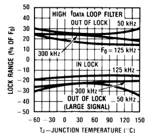
**PLL Capture & Lock Range vs Junction Temperature**
