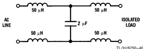
FIGURE 28. An isolation network to prevent: 1) noise from some device from polluting the AC line, and 2) to stop some low impedance device (measured at  $F_0$ ) from shorting carrier signal. Component values given as an example for  $F_0 = 125$  kHz on residential power lines
