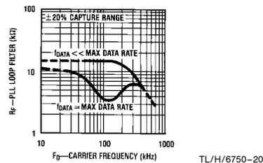
FIGURE 18. Find  $R_F$  given  $F_O$  with  $F_{\text{DATA}}$  a parameter
