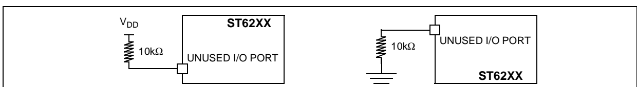
Figure 56. Two typical Applications with unused I/O Pin
