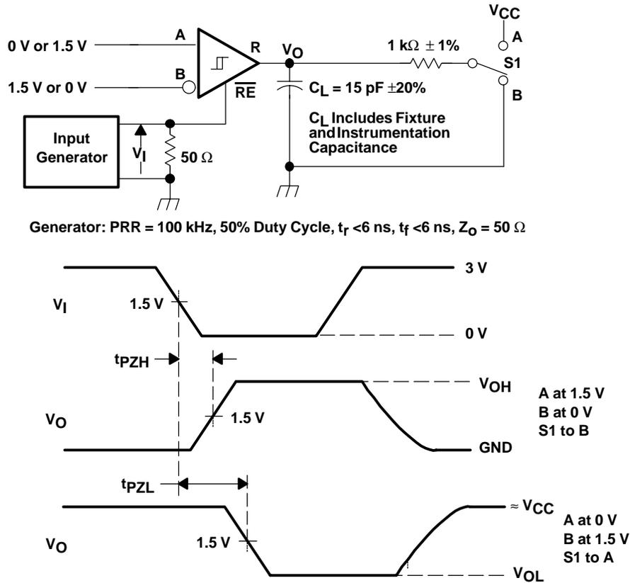
Figure 8. Receiver Enable Time From Standby (Driver Disabled)
