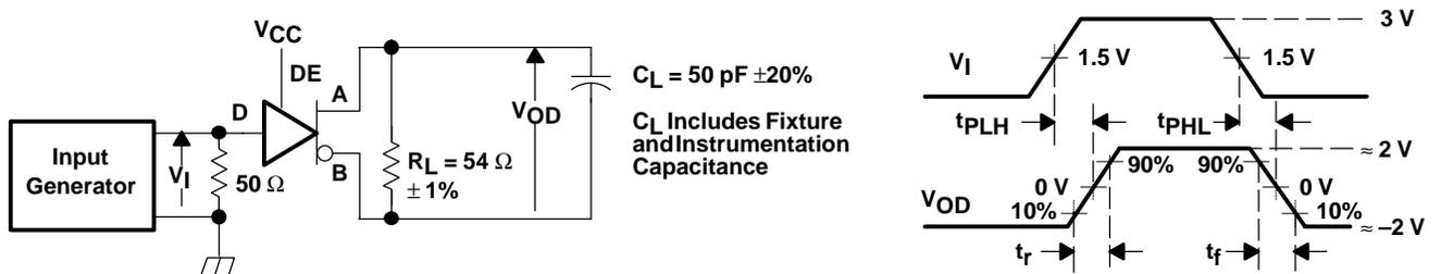
Generator: PRR = 500 kHz, 50% Duty Cycle,  $t_r < 6$  ns,  $t_f < 6$  ns,  $Z_O = 50 \Omega$
