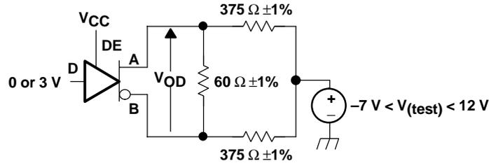
Figure 1. Driver  $V_{OD}$  With Common-Mode Loading Test Circuit
