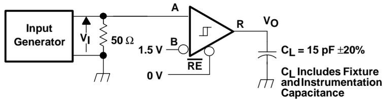
Figure 6. Receiver Switching Test Circuit and Voltage Waveforms
