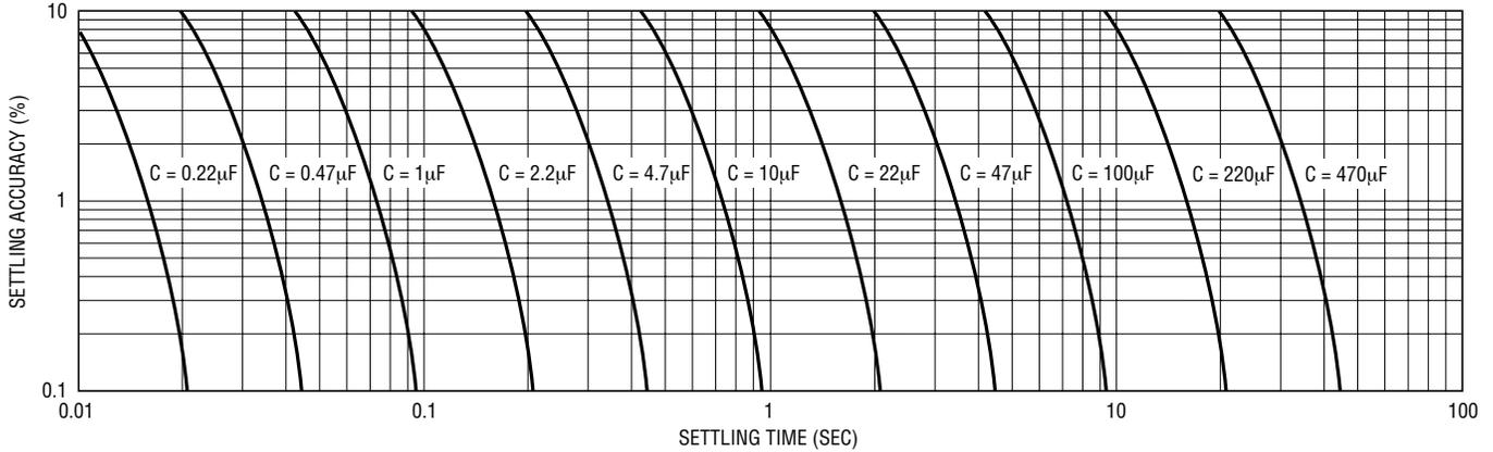
Figure 18. Settling Time with Buffered Post Filter
