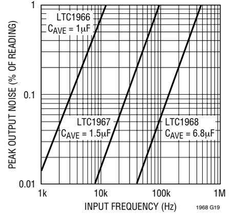
AVE CAPACITOR CHOSEN FOR EACH DEVICE TO GIVE A 1 SECOND, 0.1% SETTLING TIME
