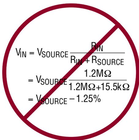
$$\begin{aligned} V_{IN} &= V_{SOURCE} \frac{R_{IN}}{R_{IN} + R_{SOURCE}} \\ &= V_{SOURCE} \frac{1.2M\Omega}{1.2M\Omega + 15.5k\Omega} \\ &= V_{SOURCE} - 1.25\% \end{aligned}$$
