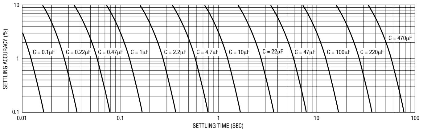
Figure 19. Settling Time with DC-Accurate Post Filter
