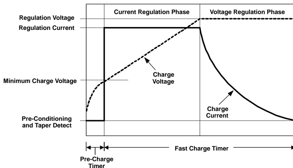
**Figure 2. Typical Charge Profile**
