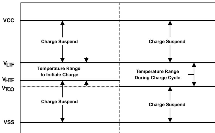
Figure 4. Temperature Sense Input Thresholds
