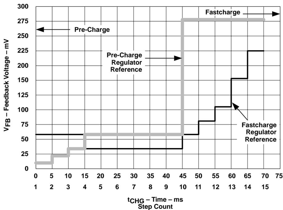
Figure 5. Typical Current Regulation Ramp From/To Pre-Charge/Fastcharge
