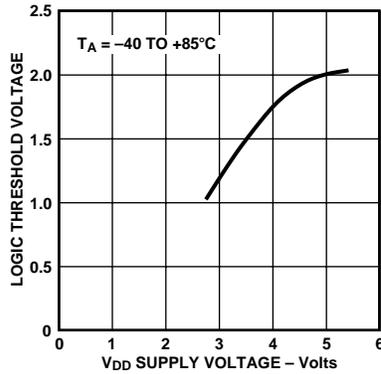
Figure 5. Logic Input Threshold Voltage vs.  $V_{DD}$
