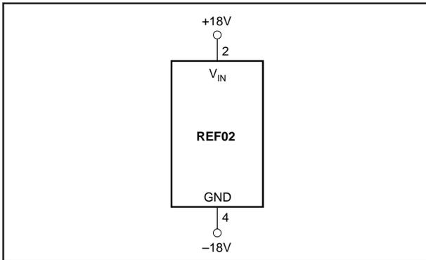
FIGURE 1. Burn-In Circuit.
