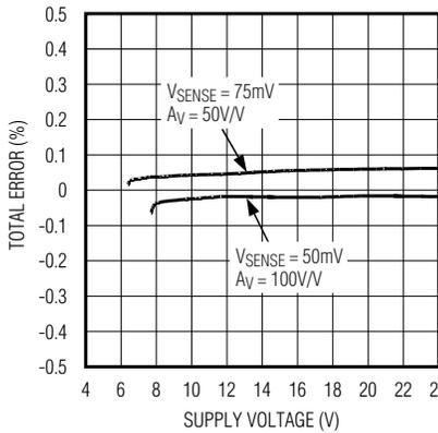
**TOTAL ERROR vs. SUPPLY VOLTAGE (VSENSE = 3mV)**
