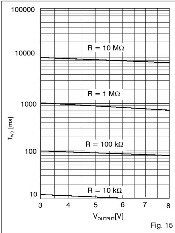
**$T_{WD}$  versus  $V_{OUTPUT}$  at  $T_J = 125^\circ\text{C}$**
