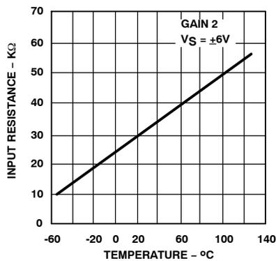
Figure 18. Input Resistance as a Function of Temperature
