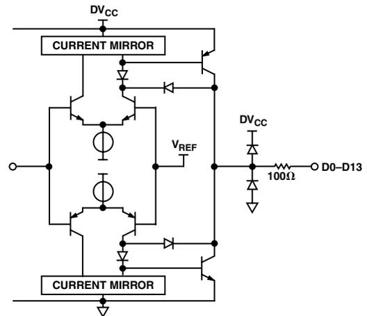
Figure 5. Digital Output Stage
