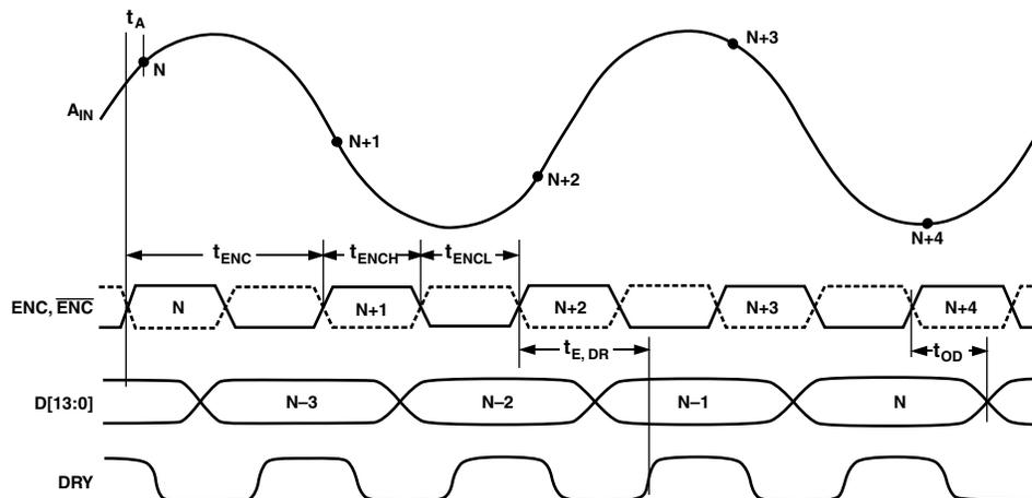
Figure 1. Timing Diagram
