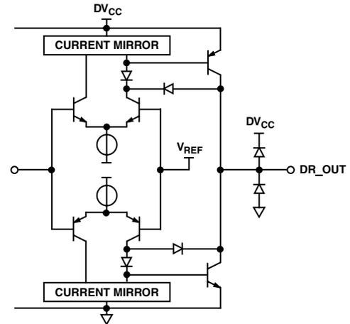
Figure 4. Digital Output Stage
