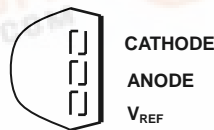
3-Pin Plastic TO-92 (Top View)
