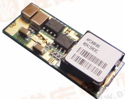
Industry Standard 0.53 X 1.3 X 0.29H SMT Package
