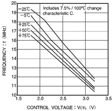
Fig. 4 Frequency vs. control voltage temperature
