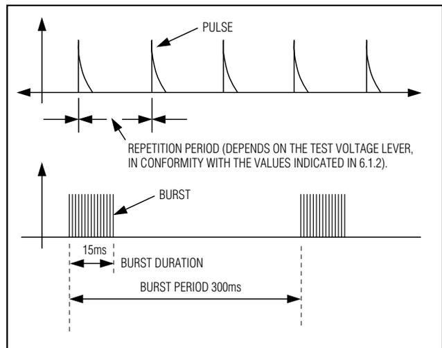
Figure 8. General Graph of a Fast Transient Burst
