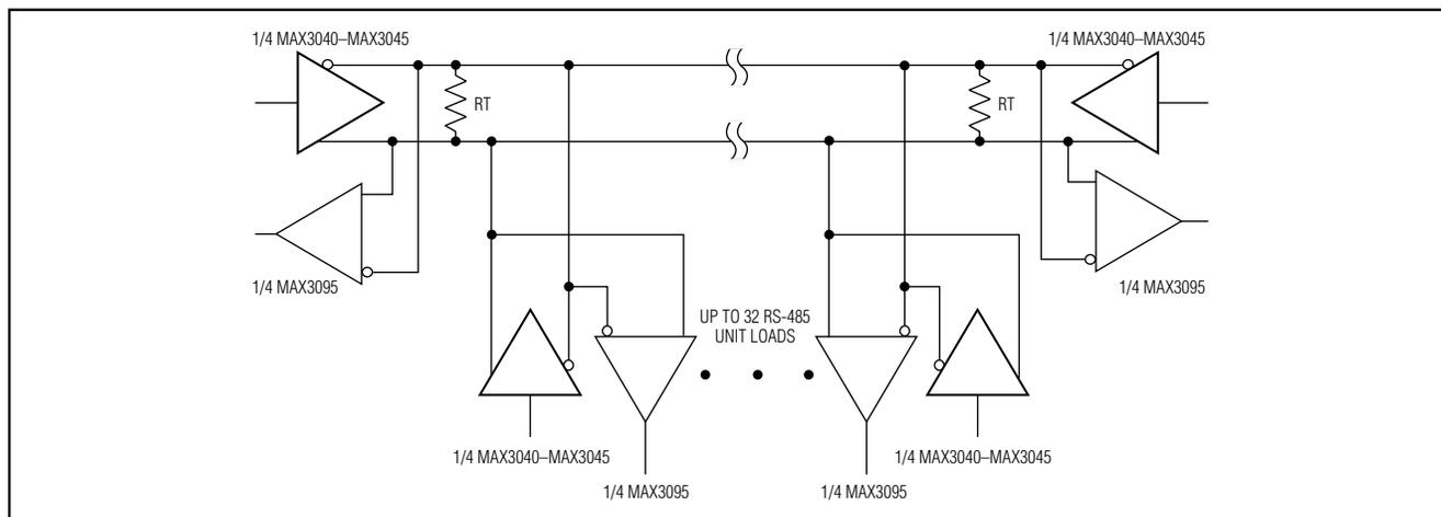
Figure 12. Typical Connection for Multiple-Point RS-485 Bus
