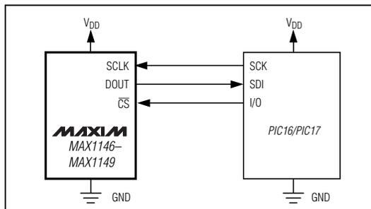
Figure 18. SPI Interface Connection for a PIC16/PIC17 Controller
