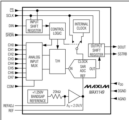
Figure 5. Functional Diagram
