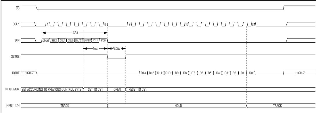
Figure 9. Internal Clock Mode Timing—24 Clocks/Conversion Timing
