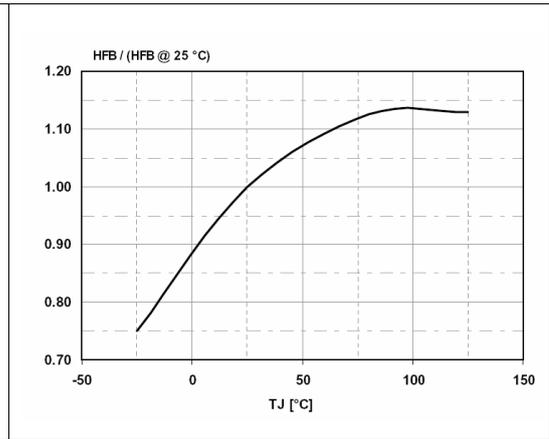
Figure 11. Brown out threshold vs  $T_J$
