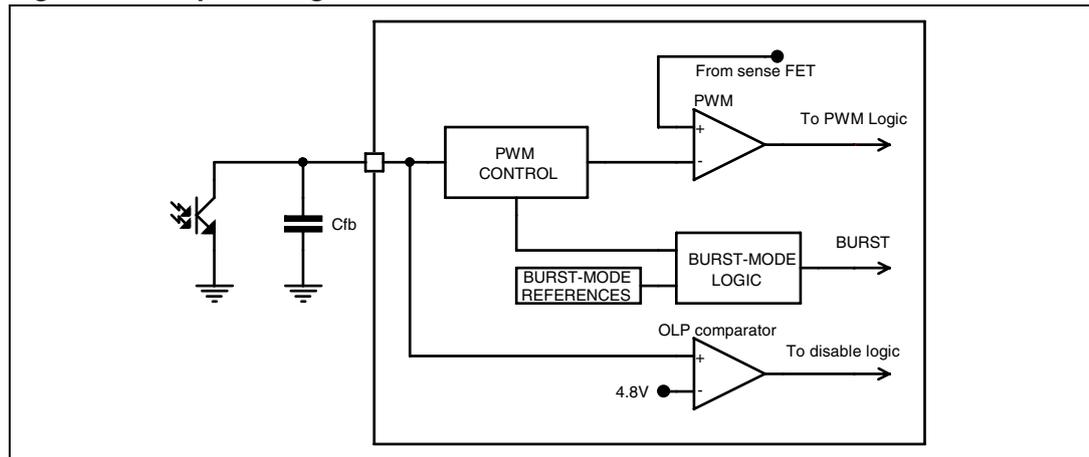
Figure 29. FB pin configuration
