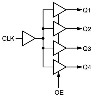
Figure 1. Block Diagram
