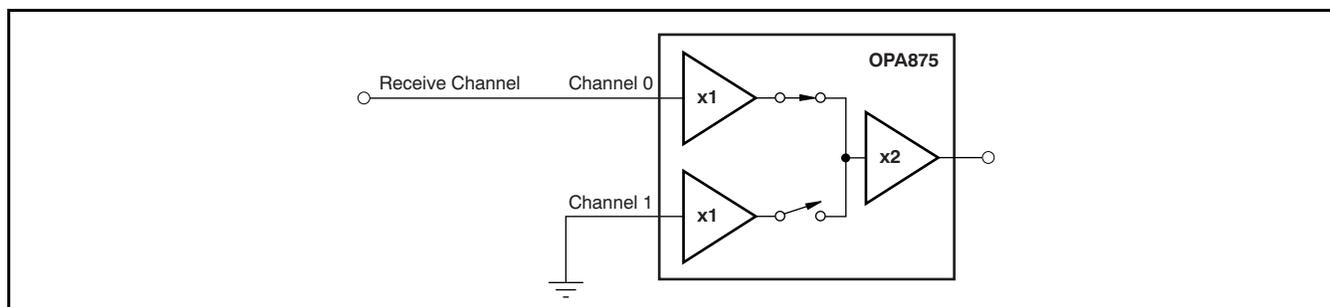
Figure 26. Transmit/Receive Switch
