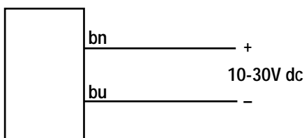
4-Pin Euro-Style Pin-out (Cable Connector Shown)
