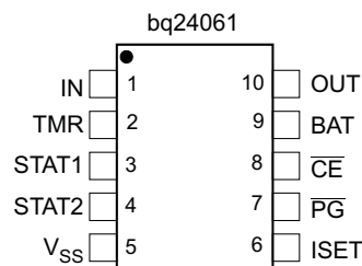
Pin Out (Top View)
