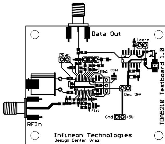
Figure 5-2 Top Side of the Evaluation Board
