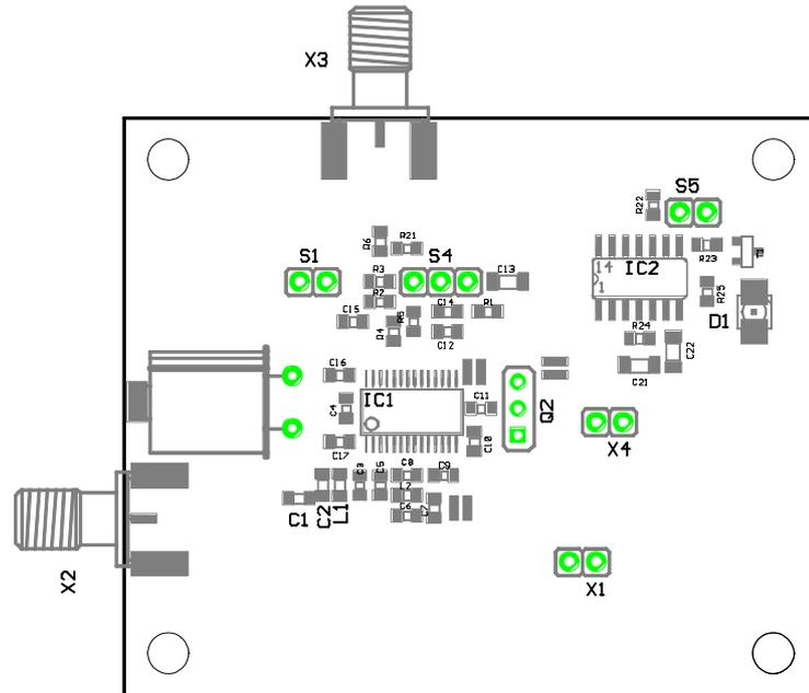
Figure 5-4 Component Placement on the Evaluation Board
