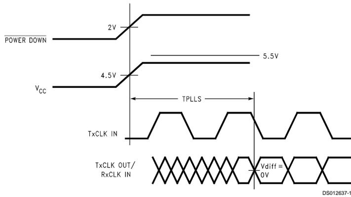
**FIGURE 10. DS90CR211 (Transmitter) Phase Lock Loop Set Time**
