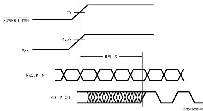
**FIGURE 11. DS90CR212 (Receiver) Phase Lock Loop Set Time**
