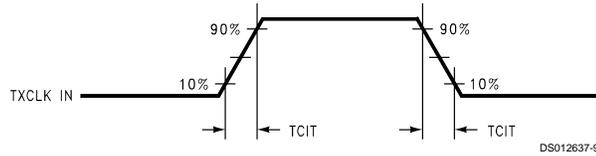
**FIGURE 4. DS90CR211 (Transmitter) Input Clock Transition Time**
