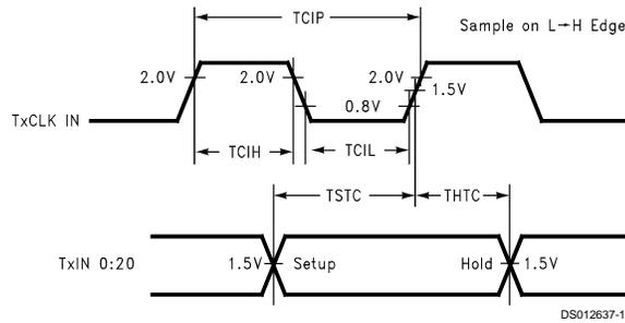
**FIGURE 6. DS90CR211 Setup/Hold and High/Low Times**
