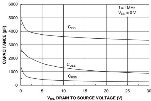
**Figure 8. Capacitance Characteristics.**
