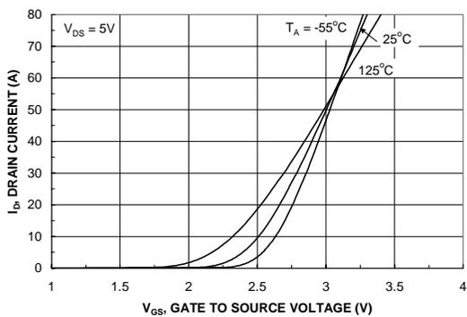
Figure 5. Transfer Characteristics.
