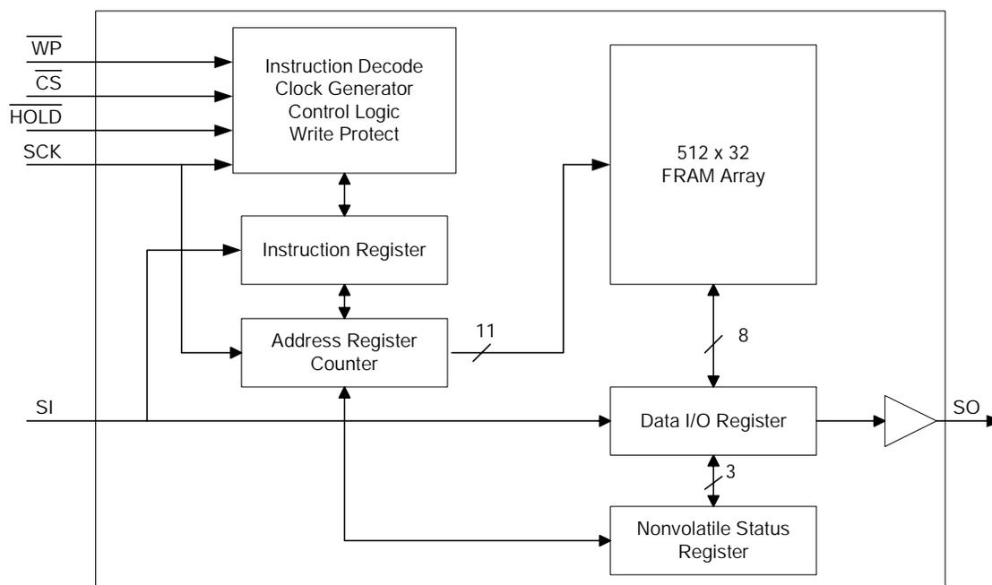
Figure 1. Block Diagram
