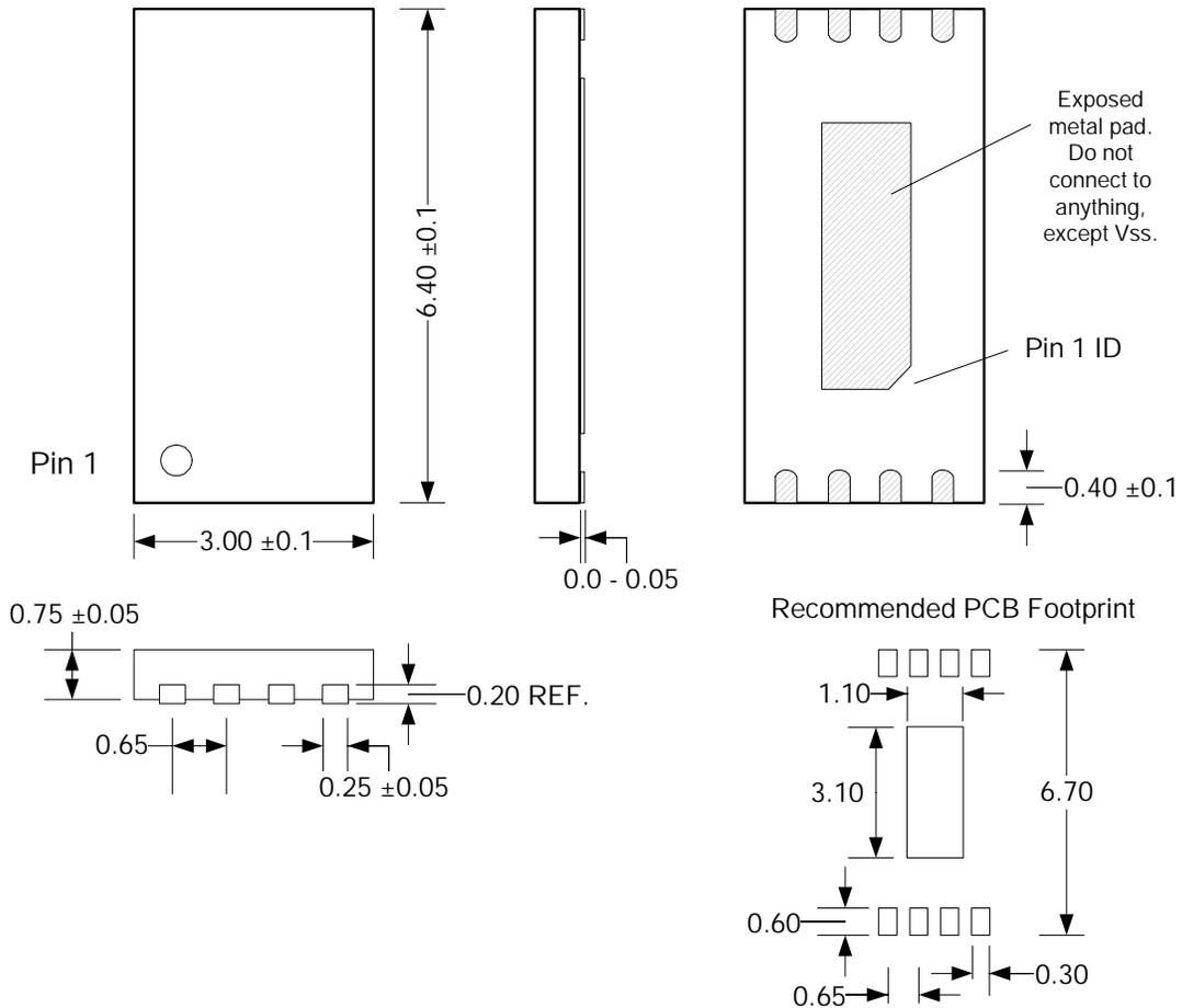
Note: All dimensions in millimeters. This package is footprint compatible with the 8-pin TSSOP.
