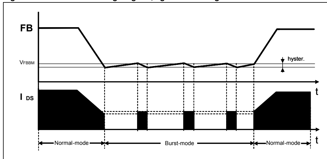
Figure 30. Burst mode timing diagram, light load management
