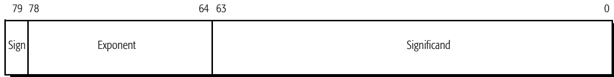
Figure 11. Floating-Point Register
