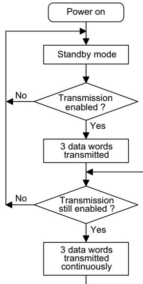
Notes: D12~D17 are transmission enables of the HT6187/HT6207/HT6247.
