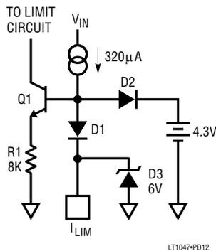
Figure 8. I<sub>LIM</sub> Pin Circuit
