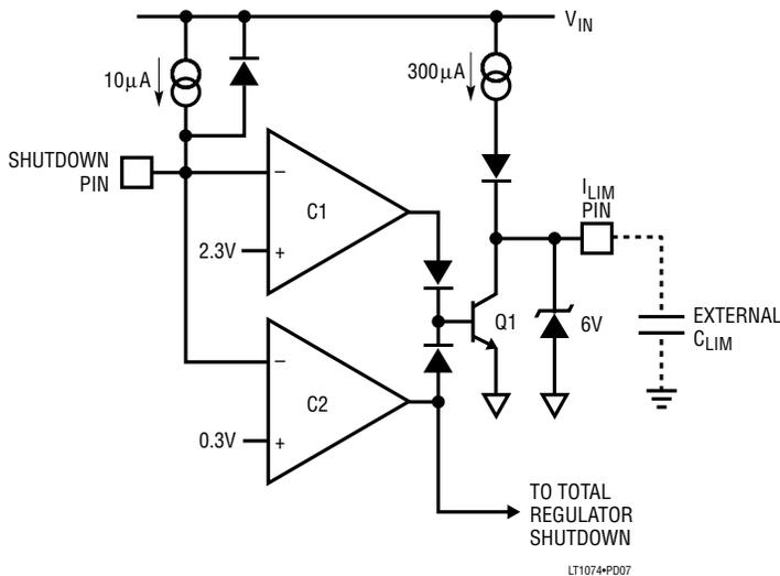
Figure 5. Shutdown Circuitry
