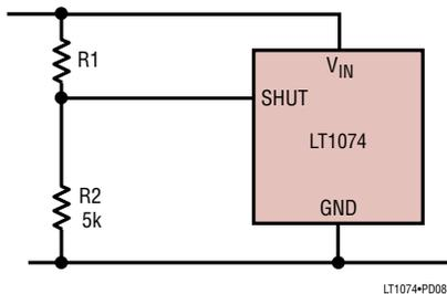
Figure 6. Undervoltage Lockout
