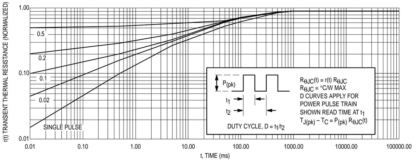
Figure 21. Typical Thermal Response ( $Z_{\theta JC}(t)$ ) for MJF18002
