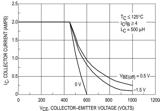
Figure 16. Reverse Bias Switching Safe Operating Area
