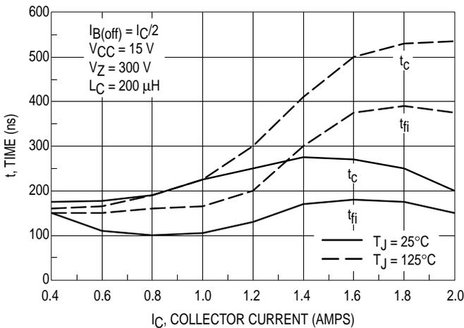
Figure 11. Inductive Switching,  $t_c$  &  $t_{fi}$ ,  $I_C/I_B = 5$
