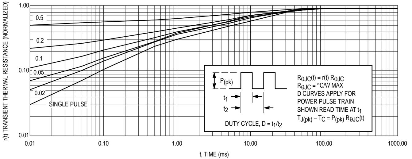
Figure 20. Typical Thermal Response ( $Z_{\theta JC}(t)$ ) for MJE18002
