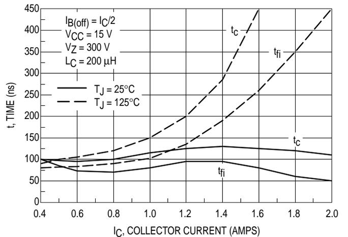
Figure 12. Inductive Switching,  $t_c$  &  $t_{fi}$ ,  $I_C/I_B = 10$
