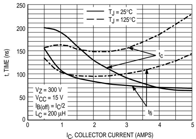
Figure 12. Inductive Switching,  $t_c$  &  $t_{fi}$ ,  $I_C/I_B = 10$
