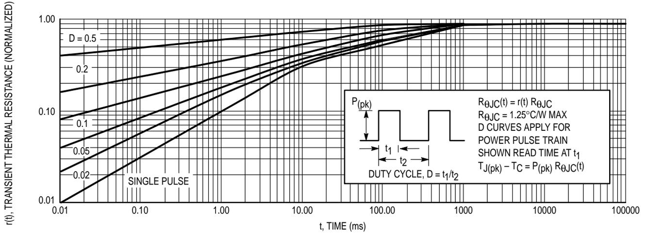
**Figure 20. Typical Thermal Response ( $Z_{\theta JC}(t)$ ) for MJE18004**
