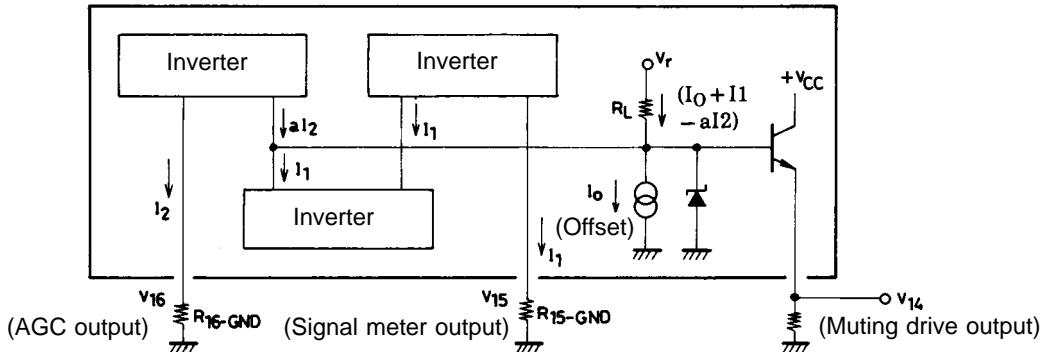
By referring to the illustration,  $V_{14}$  is given by the formula:  $V_{14} = V_r - (I_O + I_1 - aI_2)R_L - V_{BE}$ .
