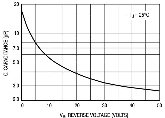
Figure 5. Typical Capacitance
