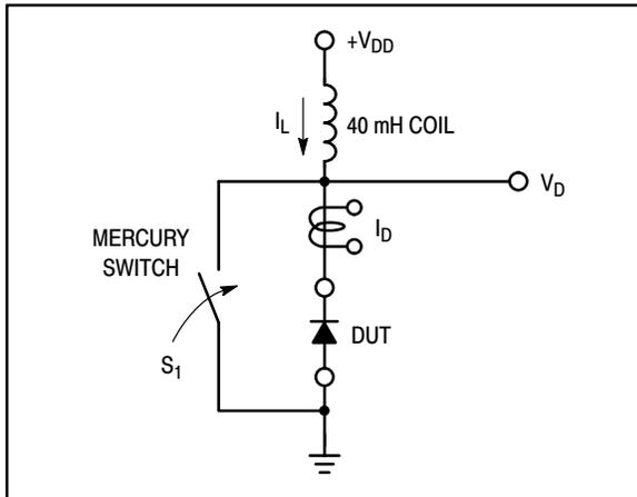
Figure 6. Test Circuit
