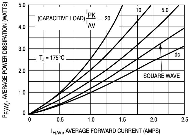
Figure 4. Power Dissipation
