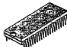
42-PIN PLASTIC SHRINK DIP (DIP-42P-M02)
