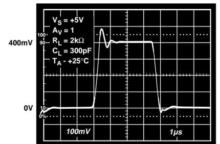
Figure 37. Small Signal Transient Response
