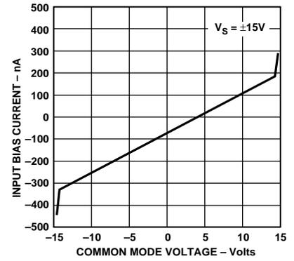
Figure 8. Input Bias Current vs. Common-Mode Voltage
