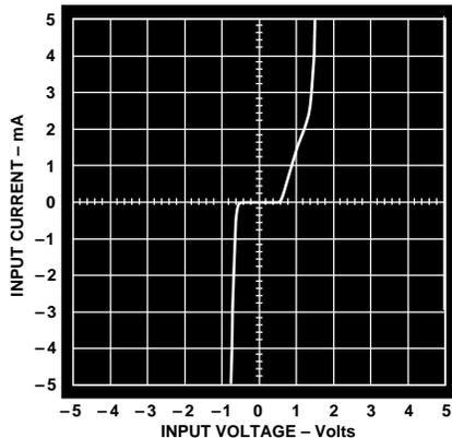
Figure 43. Input Overvoltage I-V Characteristics of the OP284
