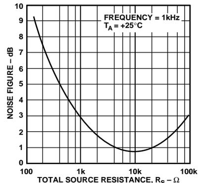
Figure 47. OP284 Noise Figure vs. Source Resistance
