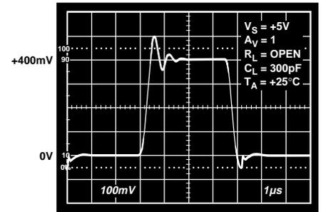
Figure 36. Small Signal Transient Response
