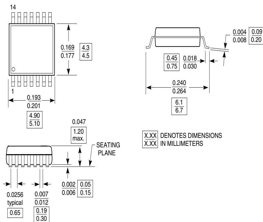
**Packaging Mechanical: 14-Pin SOIC (W)**
