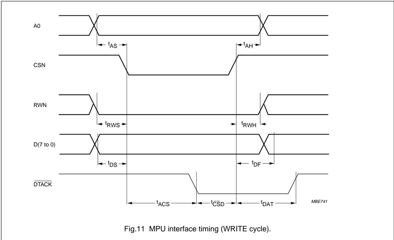
Fig.11 MPU interface timing (WRITE cycle).
