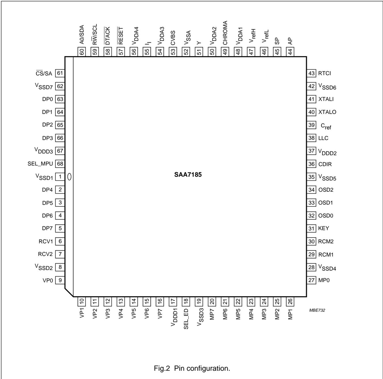
Fig.2 Pin configuration.
