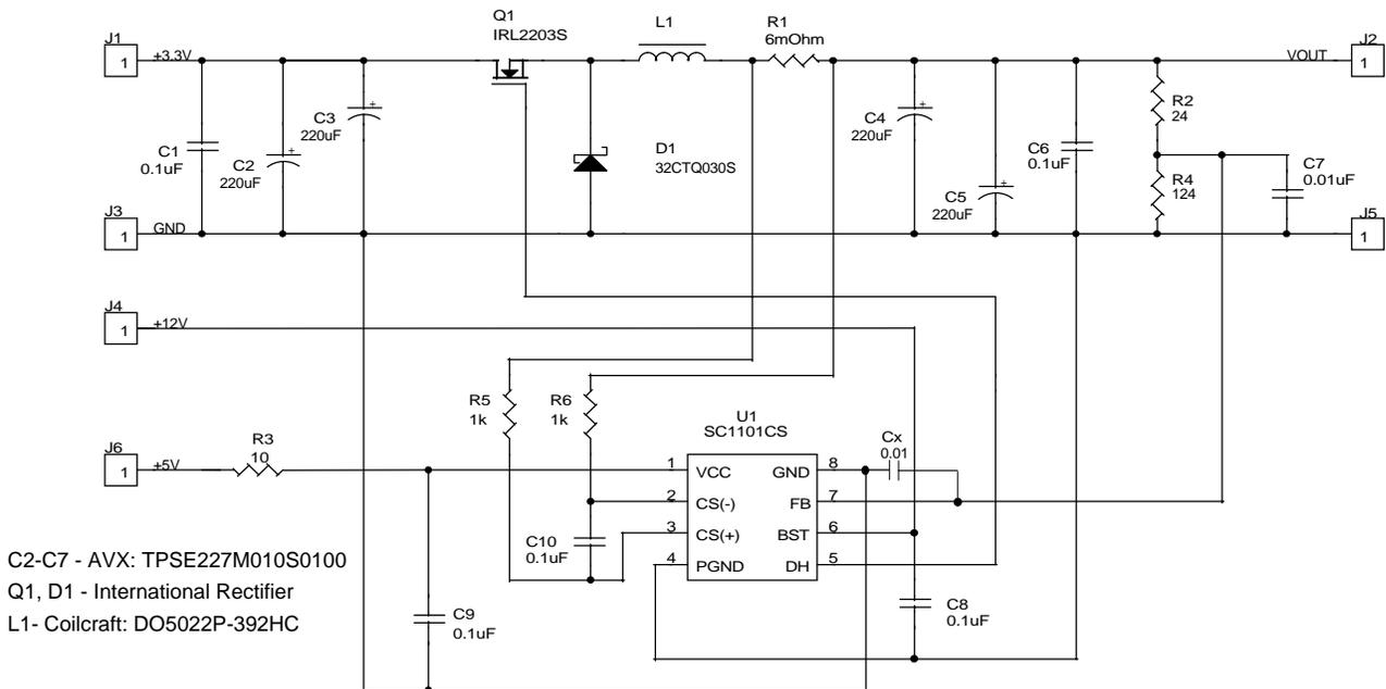
Fig. 6: GTL+ 3.3V to 1.5V 8A Application
