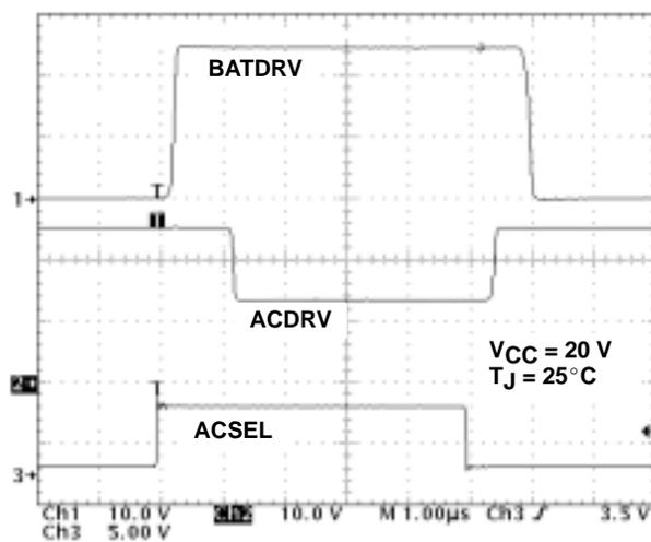
Figure 23. Power Source Select Output Break Before Make
