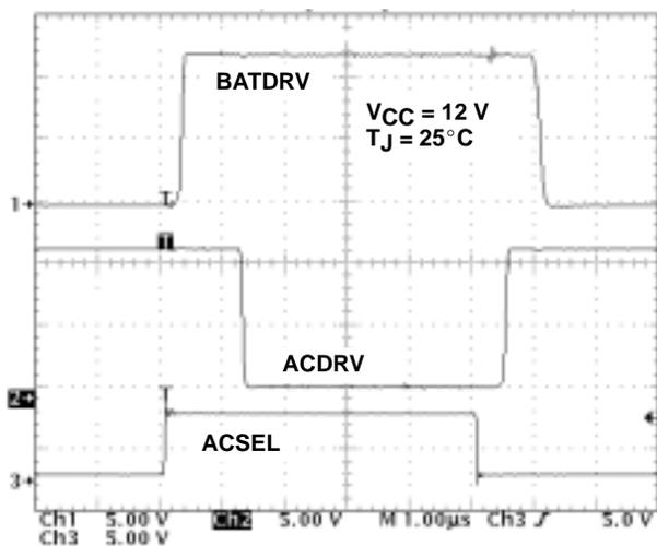
Figure 22. Power Source Select Output Break Before Make
