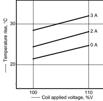
2-(2) Coil temperature rise 2 coil latching
