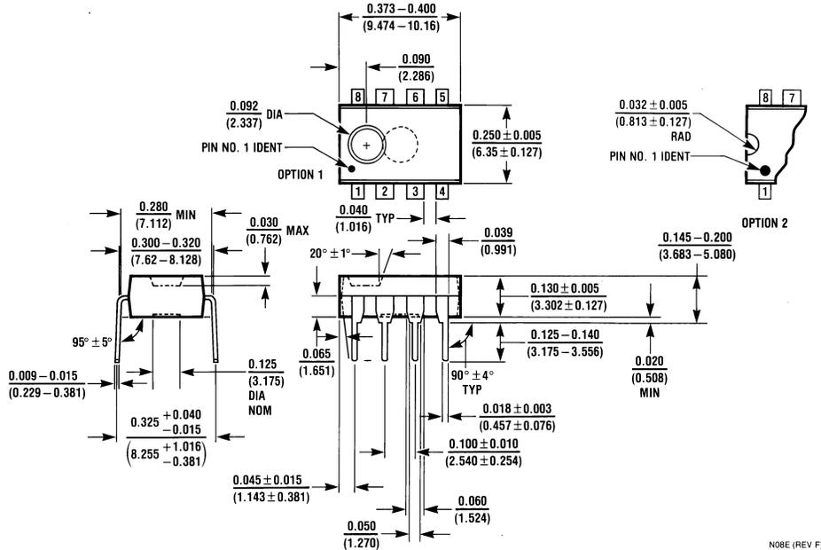
**8-Pin Molded Dual-In-Line Package**
