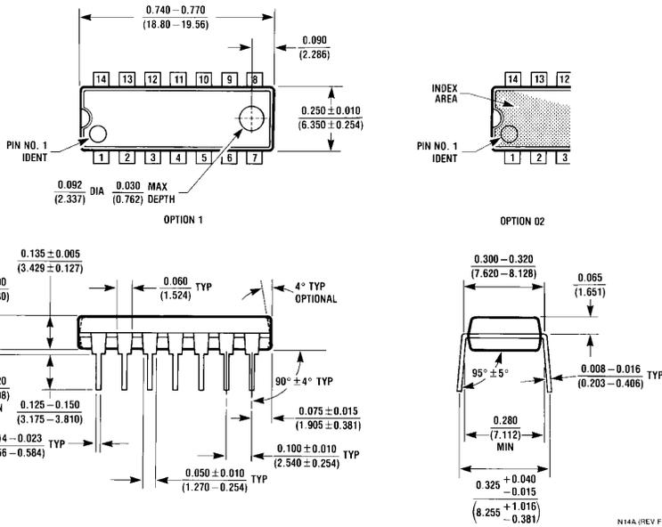
**14-Pin Molded Dual-In-Line Package**
