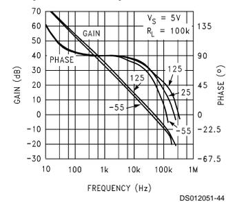
**Typical Performance Characteristics**  $V_S = +5V$ , Single Supply,  $T_A = 25^\circ C$  unless otherwise specified (Continued)
