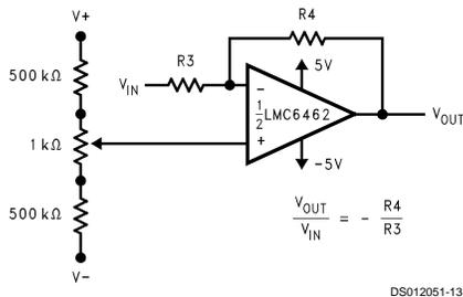
**FIGURE 9. Inverting Configuration Offset Voltage Adjustment**
