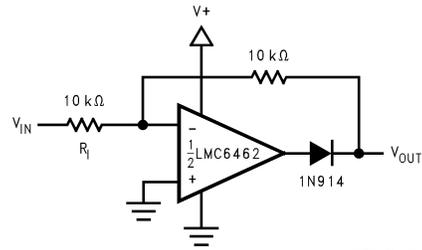
FIGURE 19. Full-Wave Rectifier with Input Current Protection ( $R_1$ )
