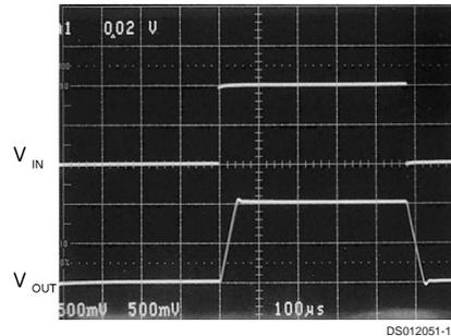
**FIGURE 7. Pulse Response of LMC6462 Circuit in *Figure 6***
