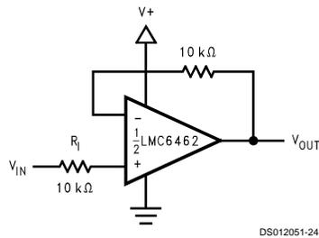
FIGURE 18. Half-Wave Rectifier with Input Current Protection ( $R_1$ )
