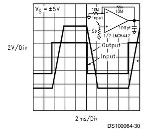
**Small Signal Step Response (AV = -1) (CL=1MΩ || 100 pF, 200 pF)**
