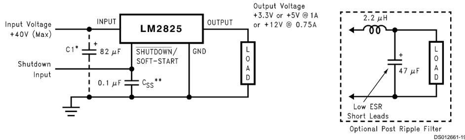
\*Optional—Required if package is more than 6" away from main filter or bypass capacitor.
