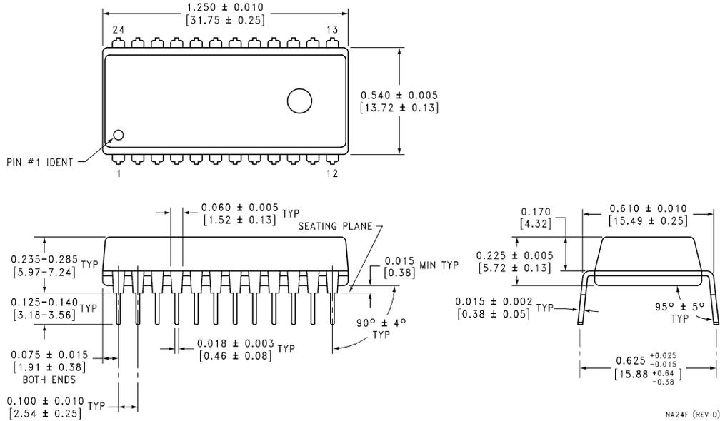
**24-Lead (0.600" Wide) Molded Dual-In-Line Package**
