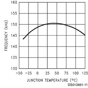
**Typical Performance Characteristics** (Circuits of Figure 2 and Figure 3) Unless otherwise specified,  $V_{IN} = 12V$  for 3.3V, 5.0V and ADJ versions,  $V_{IN} = 24V$  for 12V and H-ADJ versions,  $I_{LOAD} = 100\text{ mA}$ ,  $T_A = 25^\circ\text{C}$  (Continued)
