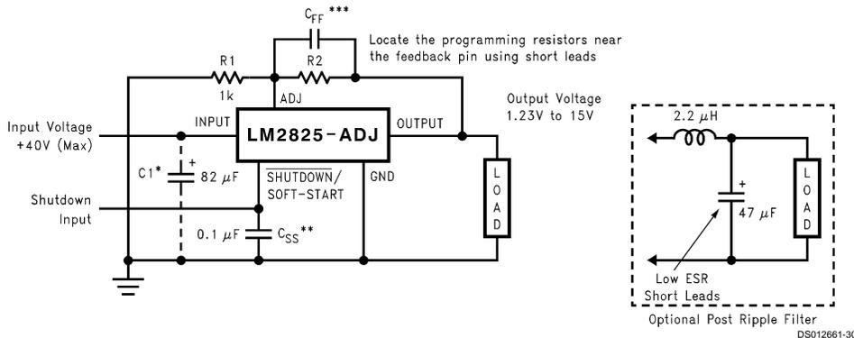
\*Optional—Required if package is more than 6" away from main filter or bypass capacitor.
