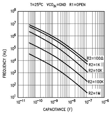
**Typical Offset Frequency vs R2, C1**  $V_{CC} = 6V$
