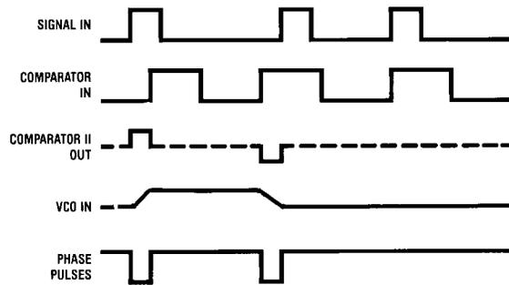
FIGURE 7. Typical Phase Comparator II Output Waveforms
