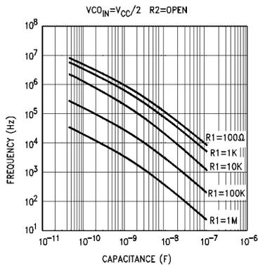
**Typical Center Frequency vs R1, C1**  $V_{CC} = 6V$
